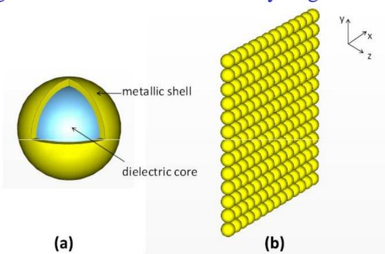
**Figure 1:** (Left) Schematic diagram of the plasmonic nanostructure which is mediated between the two qubits of our system. The two qubits are placed in same distances from the nanostructure. (a) A metal-coated dielectric nanosphere and (b) Square lattice (monolayer) of metal-coated dielectric nanospheres.
