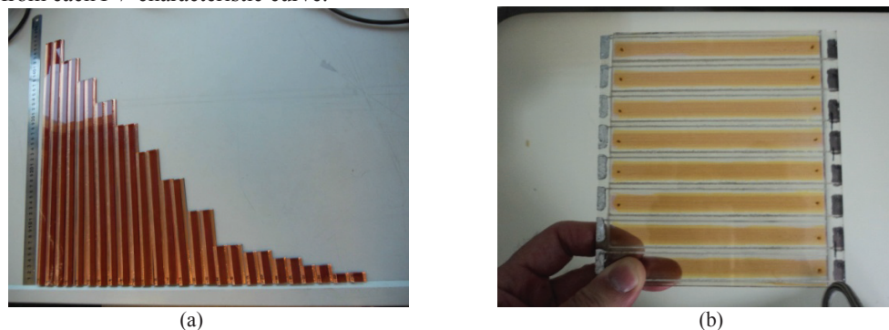
FIGURE 1. (a) Image of all strip shaped DSSCs used varied from 1 \times 1 to 1 \times 45 \text{ cm}^2 . (b) DSSC module of 20 \times 20 \text{ cm}^2
