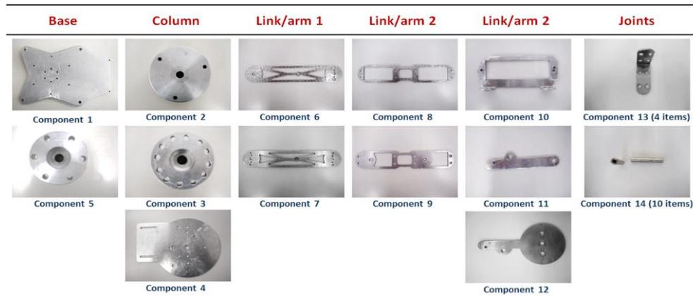
Figure 3. Numbered components of the robotic aluminium frame.
